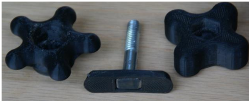
Picture #1 3D printed knobs and bolt with 3D printed wedge on bottom.
