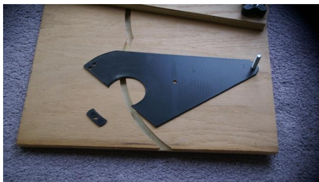
Picture #2 3D printed router jig used to cut V channels in base. Printed in 2 parts because it was too large for my printer.
